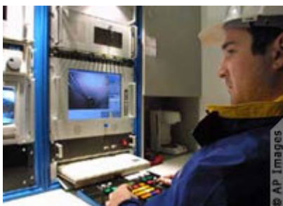
Watching real-time video from inside a sewer line, a technician maneuvers a robot through a sewer.
